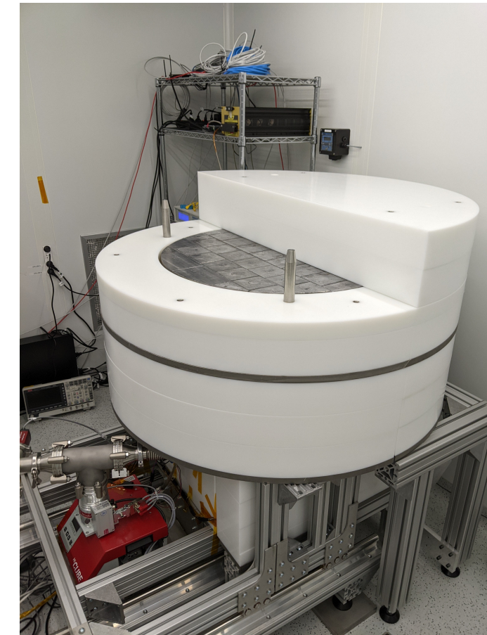
Low-background lead and polyethylene external shield in place
